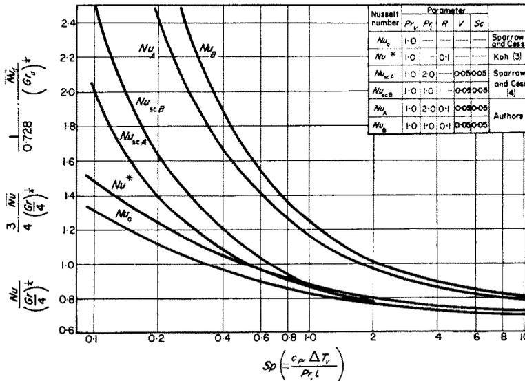
FIG. 5. Comparison of heat transfer result with the former solution.
