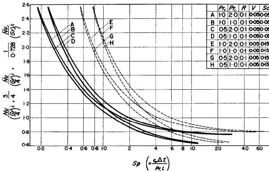
FIG. 6. Effects of Prandtl number and subcooling on heat transfer.
