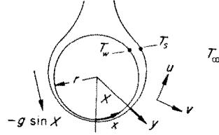
FIG. 2. Physical model and co-ordinates for horizontal cylinder.
