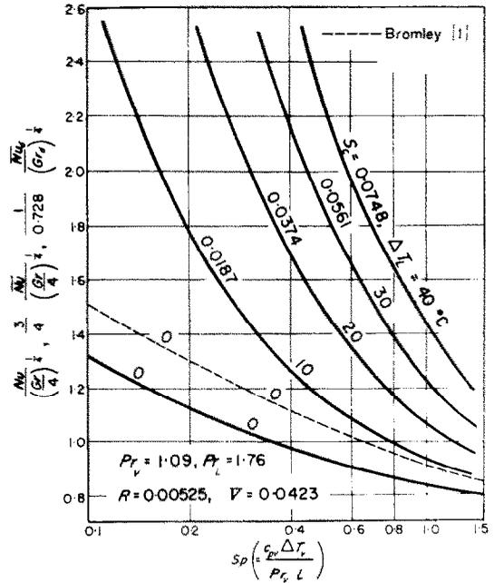
FIG. 8. Non-dimensional representation of heat-transfer characteristics of water at 1 atm.
