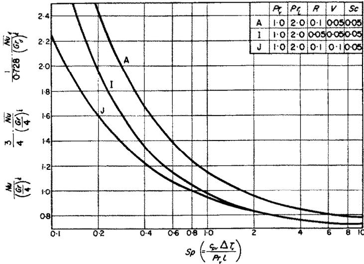
FIG. 7. Effects of  $R$  and  $V$  on heat transfer.
