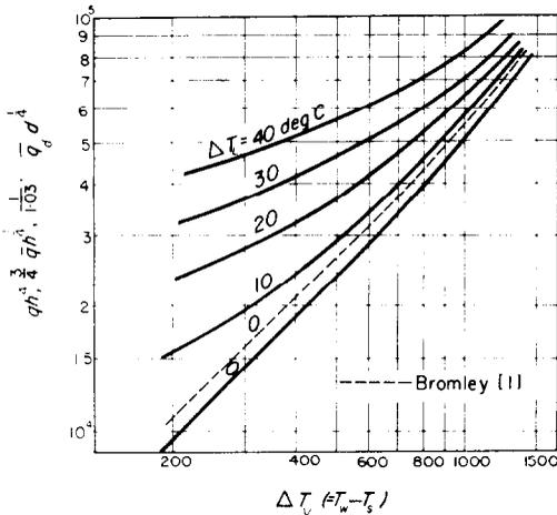
FIG. 9. Boiling curve representation of heat-transfer characteristics of water at 1 atm.
