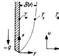
FIG. 1. Physical model and co-ordinates for vertical plate.
